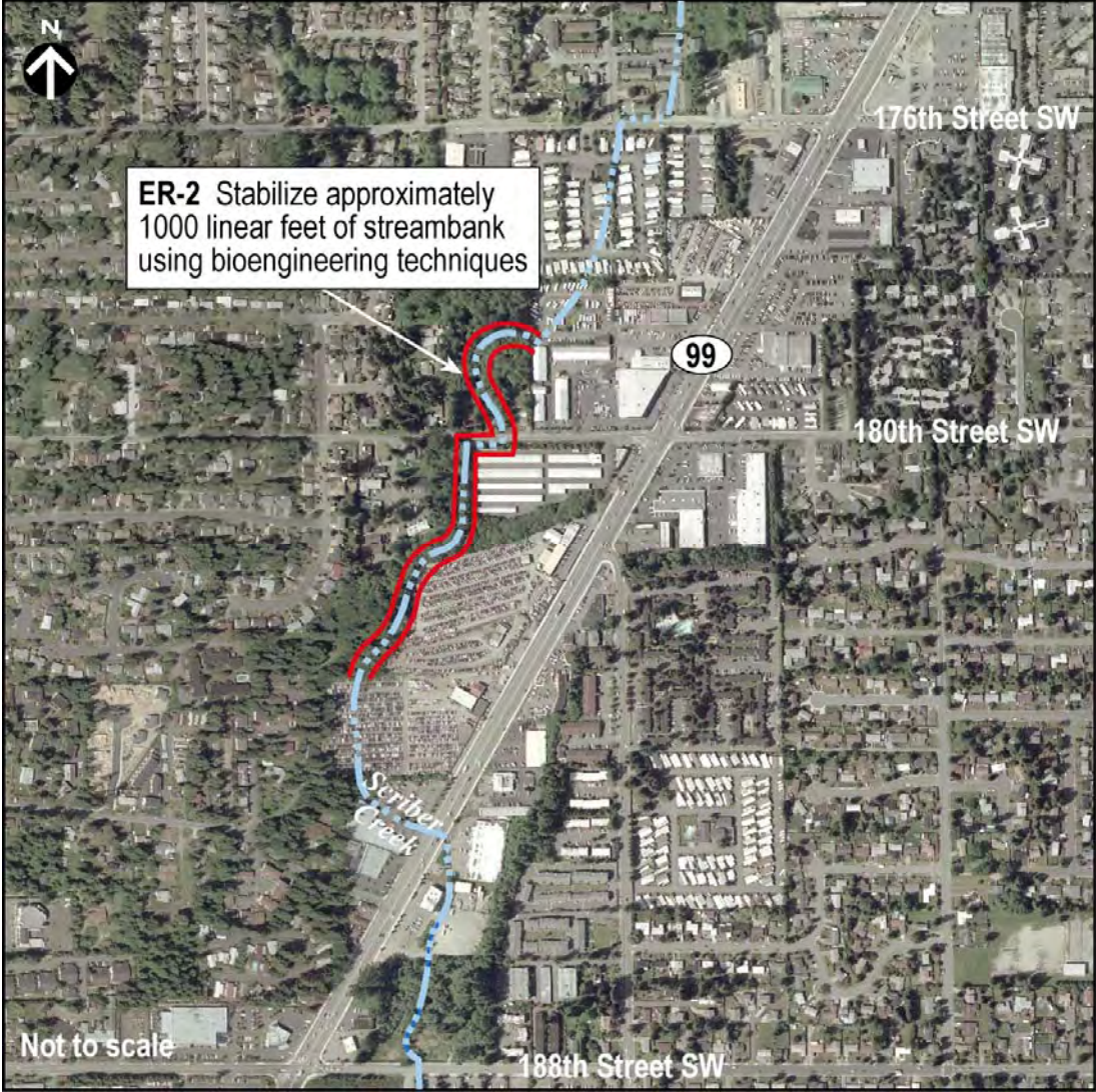
Figure 1. Proposed location for Scriber Creek bank stabilization.
