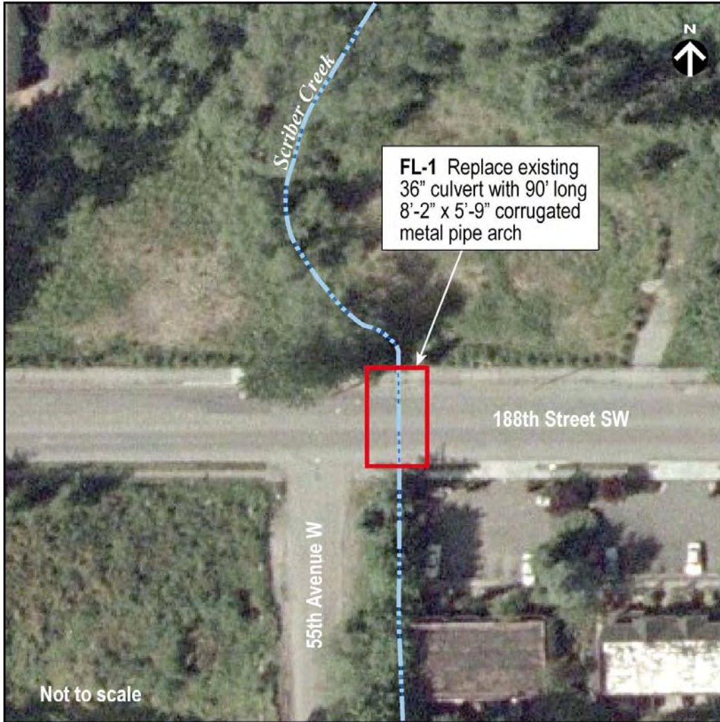
Figure 1. Proposed location for Scriber Creek culvert replacement at 188th Street SW.
