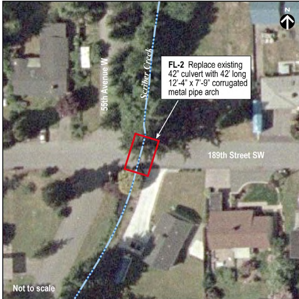
Figure 1. Proposed location for Scriber Creek culvert replacement at 189th Street SW.
