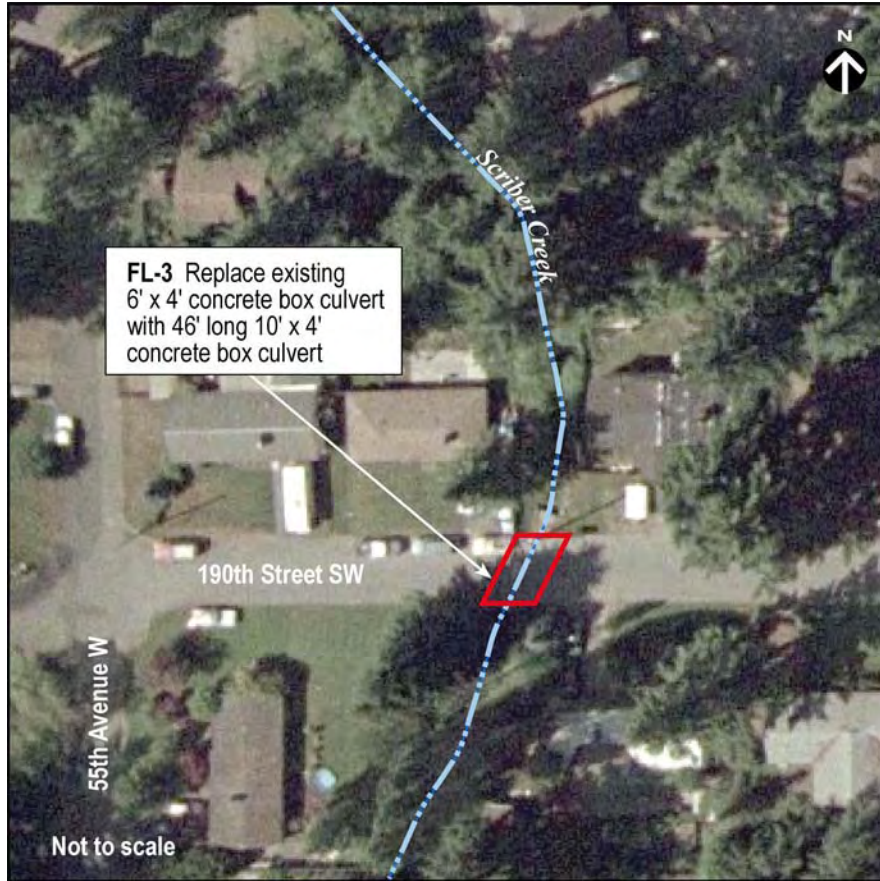
Figure 1. Proposed location for Scriber Creek culvert replacement at 190th Street SW.
