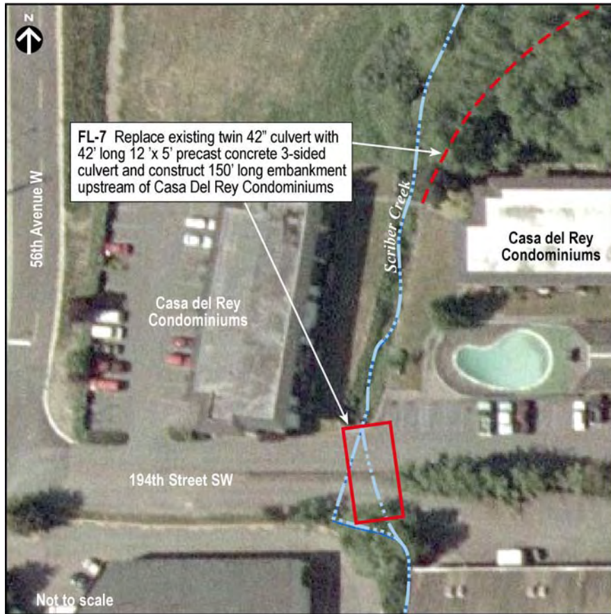
Figure 1. Proposed location for Scriber Creek culvert replacement at Casa Del Rey condominiums driveway.
