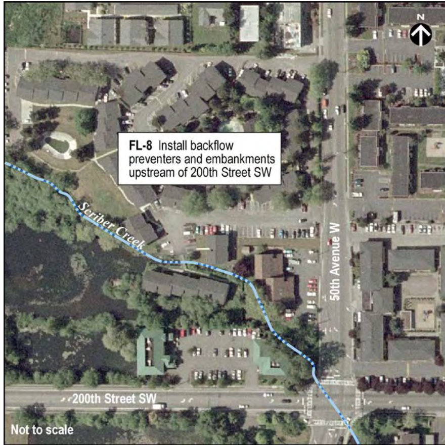
Figure 1. Install backflow preventers on storm drain outfalls and construct embankments along Scriber Creek upstream of 200th Street SW and 50th Avenue W.
